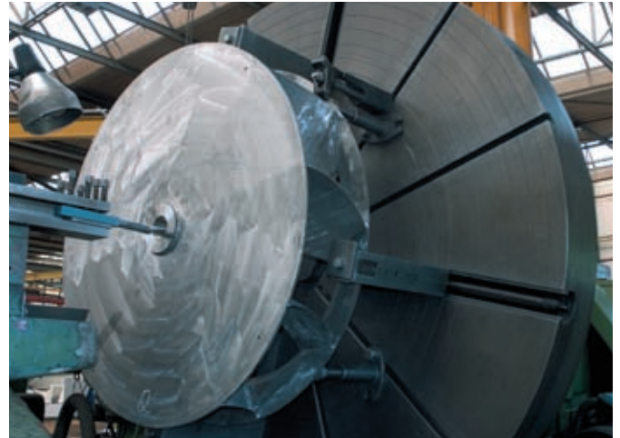
Blower impeller processing on a heavy-duty lathe
