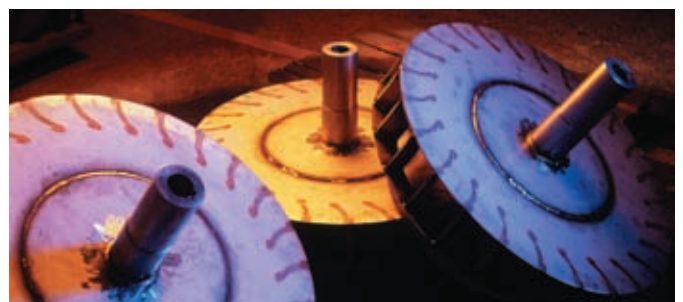
Circulation fan for strip suspension system (650 °C)
